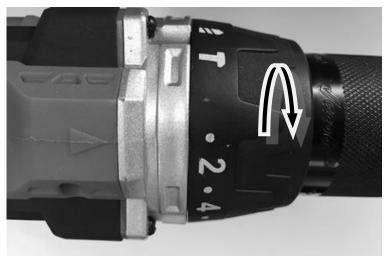
When the selected torque is reached, the chuck will stop rotating. The proper setting depends on the type of material and the size of screw you are using.
