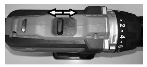
Use the low speed (1) for high power and torque applications and high speed (2) for fast drilling or driving applications.
